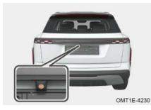
Installation position of rear camera: located on center part above rear license plate.
