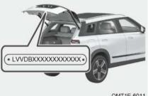
Vehicle Identification Number (VIN) label is located on back door as shown in the illustration.
