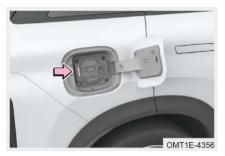
The indicator light strip is located inside the charging port cover.
