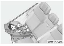
A rearward facing child restraint is installed to face to the rear of the vehicle. Only install a rearward facing child restraint on the front passenger seat if the airbag is OFF. It is recommended children use a rearward facing child restraint system up to 4 years old.
