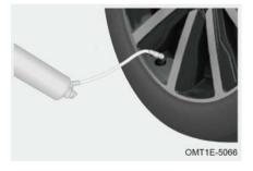
Step 3: Tighten the junction valve of the automatic inflation tire repair liquid to the tire valve;
