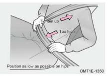
To adjust the seatback angle, sit up straightly and well back in the seat. Position the lap belt as low as possible on your hips - not on your waist, then pull the shoulder section upward so that it comes fully over the shoulder, but does not come into contact with the neck or slide off the shoulder.
