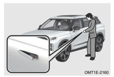
Step 2: Pull the door handle, insert the mechanical key into the keyhole door handle. inside the turn clockwise to lock the door. counterclockwise to unlock the door.
