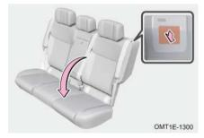
Adjust height of seat head restraints, remove them if necessary and fold up center armrest. Then pull the left seatback adjustment handle forward and pull seatback forward to fold it down slowly. This can enlarge the luggage storage space.
