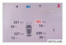
When tire pressure is less than 192 bar and speed is no lower than 25 km/h for a period of time, system will send a low pressure warning, corresponding wheel symbol will blink, current tire pressure value will be displayed and " (!) " yellow indicator in instrument cluster will remain on.
