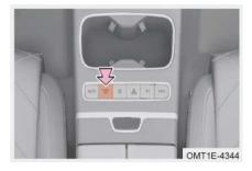
With vehicle in READY state, press "MORE" button to cycle through the driving modes; The corresponding mode indicator on instrument cluster comes on, accompanied by voice reminder, to prompt you that driving mode is switched successfully.
