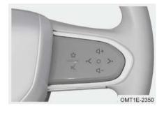
Customization button "  $\overleftrightarrow$  ": This button can be customized in audio system - Vehicle Center - Vehicle Settings.
