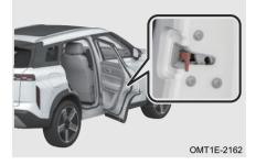
Vehicle cannot be locked electrically when battery is depleted or under similar conditions, in this case, the doors can be locked with emergency locking function.
