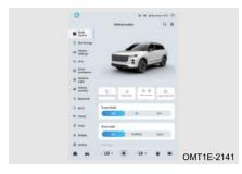
With vehicle in READY state, click central locking button through Audio System - Vehicle Center -Quick Control to unlock/lock doors.
