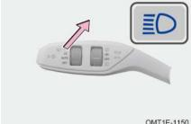
When turning on low beam light, pull headlight combination switch away steering from wheel side and release, headlight high beam comes on; Pull headlight combination switch towards steering wheel side and release to turn off headlight high beam.
