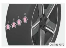
Check the tire tread by tread wear mark. When tread wear reaches its limit, tread will be in the same plane as the wear band. If such condition occurs, the tire performance and safety will be seriously impacted, and replacement is necessary.
