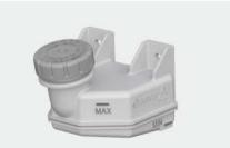
Brake fluid level should be between the "MIN" and "MAX" marks. If the level is at or below the "MIN" mark, add brake fluid and contact the authorized service station for inspection and repair immediately.
