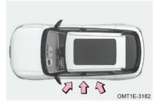
The vehicle is subjected to a strong side impact, and the side collision sensors detect an impact severe enough to cause the side airbags, curtain shield airbags, and front middle airbag to deploy.
