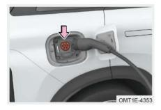
Step 4: Open the back door and take out the charging device, then insert the three-pin plug into a standard power socket (only using on-board charging gun is applicable to this step). If AC charging pile is used for charging, please skip to step 5 directly:
