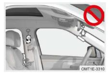
Do not attach anything to areas such as the door, windshield glass, side door glass, A pillar, B pillar, C pillar, roof side rail and assist grip.
