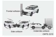
The driver airbag, front passenger airbag and driver knee airbag (if equipped) may not deploy if the front of vehicle hits a telegraph pole, goes under a truck, or if the vehicle is involved in an sideways collision.
