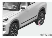
Step 2: Fit wheel bolt wrench to wheel bolt of flat tire, set the handle on left side, hold the end of wrench handle and push it downward, loosen each bolt of flat tire about one-half turn;
