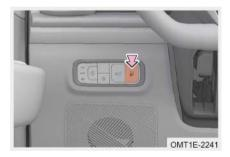
Step 1: The vehicle is parked, long press " I button and instrument cluster displays "It is ready to refuel, please refuel" message, and fuel tank cap unlocks after the pressure relief is completed;
