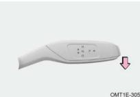
Step 1: Depress the brake pedal completely and shift the shift lever to D; Manually or automatically release the park brake and release the brake pedal to drive the vehicle slowly.
