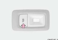
Press rear dome light switch, the light comes on, press the switch again to turn off light.
