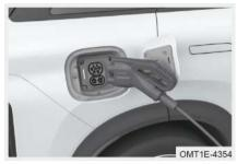
Charging gun has anti-theft function. After inserting charging gun and entering full power charging or when doors are locked, charging gun will be locked automatically. **RESCUE INFORMATION**
