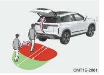
While vehicle power is switched to OFF mode or vehicle is started remotely, four doors are closed, approach to the back (red area) of vehicle when carrying smart key on your person and wait 3 seconds, after turn signal lights come on, take a step back (green area), power back door opens.
