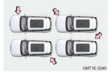
The side airbags, curtain shield airbags and front middle airbag may not deploy if the vehicle is subjected to a collision from side, the rear part of the rear tire or a side collision at certain angles to the vehicle.
