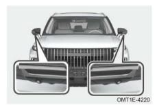
Installation position of left / right cameras: located at the bottom of left / right outside rear view mirrors.
