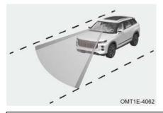
When vehicle speed is no less than 65 km/h and lane line is recognized, LDP enters standby status.
