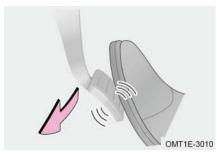
With vehicle powered on, carry the smart key on your person and enter the vehicle, depress brake pedal to start vehicle, and "READY" green indicator on instrument cluster remains on.
