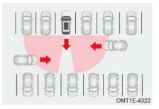
Shift the shift position to R and vehicle speed is less than 15 km/h, rear traffic crossing anti-collision system is activated; In other gear positions, system is in standby status.
