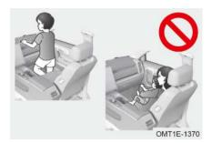
Make sure the shoulder belt is positioned across the center of child's shoulder. The belt should be kept away from child's neck, but not falling off child's shoulder. Otherwise, the child is at risk of serious injury or even death during a collision.
