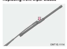
Step 1: Click "  $4_{VFF}$  " button in control center, short press the left button of wiper switch to enter maintenance mode within several seconds after switching vehicle to power off state;
