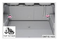
This model is equipped with top tether strap anchorages on the back of the rear seats.
