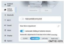
With vehicle in READY state. Set rear view mirror automatic adjustment in reversing to OFF/both sides/only the left /only the right through Audio System - Vehicle Center - Vehicle - seat / rear mirror position.
