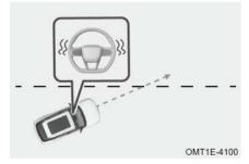
When vehicle speed is no less than 65 km/h and lane line is recognized, LDW enters standby status.
