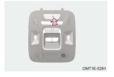
Manual activation: When required to report a serious accident, or require emergency help, long press the SOS button for 2 seconds.
