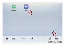
■ Entering panoramic view monitor When vehicle is in READY state, and vehicle speed is 30 km/h or less:
