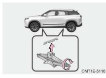
Step 3: Place jack on firm and level ground, turn jack handle clockwise by hand, making the notch of jack contact with the correct jacking-up point.
