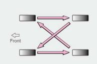
To equalize tire wear and extend tire service life, we recommends that you should rotate your tires approximately every 10,000 km (best adjustment range is 5,000 - 7,000 km); the tire rotation cycle may vary according to your driving habits and road surface conditions.
