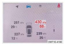
When tire temperature is higher than 85° C and speed is no less than 25 km/h for a period of time, system will send a high temperature warning, corresponding wheel symbol will blink, current tire temperature value will be displayed and "(!)" yellow indicator in instrument cluster will remain on.
