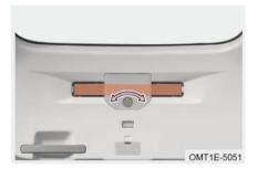
Warning triangle is located on the back door panel, turn the retaining clamp counterclockwise to remove it.
