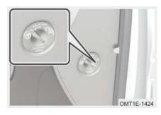
The airbag enabling/disabling switch is located on the passenger side instrument panel and is visible when front passenger door is opened.
