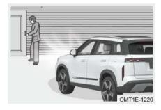
ON: With vehicle powered off, turn on the headlight auto mode before stopping. When the vehicle is in a dim environment, press lock button on smart key, and the vehicle is armed successfully. Low beam lights automatically come on for 10 seconds. Press lock button on smart key to activate it again. OFF: With vehicle powered on, turn off the headlight or reaches the set operating time, the follow me home function will turn off automatically. Low beam liahts will ao off immediately.
