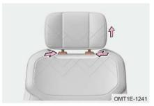
Installing head restraints: Align the head restraint with the installation holes and push it down to lock position. Press and hold the lock release button when lowering the head restraint.
