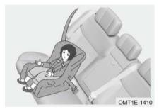
A forward facing child restraint is installed to face to the front of the vehicle. It is recommended children use a forward facing child restraint system when older than 4 years old.
