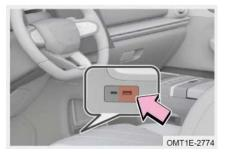
Step 3: Connect USB port and phone using original data cable; Note: Only USB port " 🕞 " supports Apple CarPlay screencast function.
