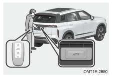
Method 1: With central control lock unlocked, approach the back of vehicle and press exterior switch, on the back door, turn signal lights will come on and power back door will be opened/closed.
