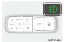
With vehicle in READY state, when position lights turn on, operate fog light switch to " <sup>\$D</sup> " position to turn on front fog lights; Turn vehicle power to OFF mode or operate fog light switch to "OFF" position again, front fog lights turn off.
