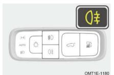
With vehicle in READY state, when front fog light or low beam lights turn on, operate fog light switch to "  $0^{\ddagger}$  " position to turn on rear fog light; After turning vehicle power to OFF mode or operate fog light switch to "  $0^{\ddagger}$  " or "OFF" position again, rear fog light turns off.
