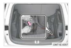
When abnormal lock fault occurs in electronic lock of the charging gun or discharging gun, the charging gun and discharging gun can be manually unlocked with electronic lock cable.
