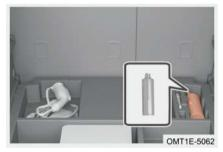
Step 1: Open back door, lift the luggage compartment carpet and take out the automatic inflation tire repair liquid;
