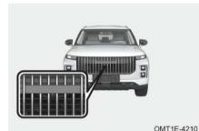
Installation position of front camera: located at intake grille of front bumper.
