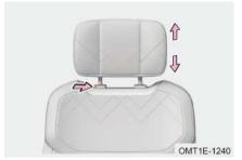
Adjust head restraint upward: Pull it up directly to a proper height.
