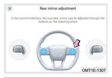
With vehicle in READY state, Audio System - Vehicle Center - Vehicle Comfort - Rear mirror adjustment.
