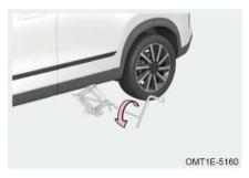
Step 2: When installing wheel bolts, screw into all wheel bolts clockwise by hand. Then straighten the spare tire, and pretighten all wheel bolts with wheel bolt wrench:
