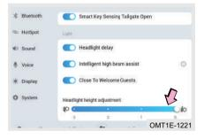
With vehicle in READY state, turn on the headlight leveling adjusting through Audio System - Vehicle Center - Quick Control.
