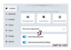
With vehicle in READY state, turn on the easy seat access/exit through Audio System - Vehicle Center -Vehicle Comfort.
