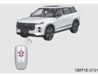
Perform unlocking operation of door to exit locking mode.
