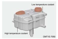
When engine is cold, the coolant level should be between the "MIN" and "MAX" marks. If the level is at or below the "MIN" mark, add coolant and contact the authorized service station for inspection and repair immediately.
