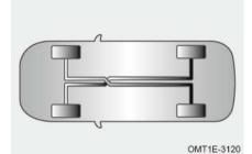
The brake system adopts X type arrangement, double circuit brake system; The system is a hydraulic with independent system two subsystems. If one of the subsystems fails, the other system can still perform brake function. However, the brake pedal should be depressed more firmly than usual and distance will the braking increase, and the brake system malfunction indicator remains on
