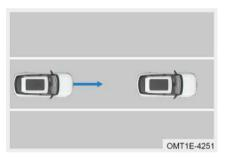
Activation conditions: The vehicle shift position is not in R and the vehicle speed is 15 km/h or more.
