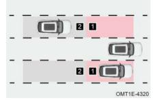
When speed increases to 15 km/h or more, BSD system enters activating; When speed is decreases from more than 15 km/h to 10 km/h, BSD system enters pre-activating.
