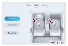
After starting the vehicle, click front seat heater button by air conditioning display screen - seat - heating, it is 3level heating (3 indicators on). Each time the switch is clicked, the heating level is lowered one level. Click it the fourth time to turn off the seat heating.
