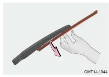
Step 1: Click "  $\mathcal{K}_{FF}$  " button in control center, push the rear wiper roller to "ON" position to enter maintenance mode within several seconds after switching vehicle to power off state;
