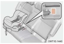
Step 2: Please press the PUSH position to access the anchorages; Step 3: Place the child restraint system on the rear outboard seat; Step 4: Attach the child restraint ISOFIX probe to the anchorage. Where necessary extend the child restraint support leg.
