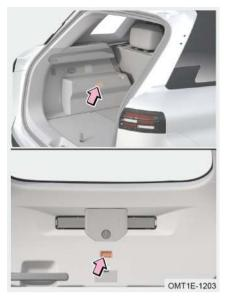
When back door is opened, luggage compartment lights will turn on for several seconds automatically. When back door is closed, luggage compartment lights will turn off immediately.
