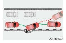
When multi-collision brake the system detects that the vehicle has collided. electronic stability the control performs svstem active braking, and decelerates the vehicle to prevent the vehicle from being collided again. In the process of braking, it can still maintain control of the vehicle, which can further ensure the safety of yourself and passers-by.
