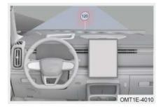
After SLA detects speed limit sign information on road in front and combines the information with speed limit information of navigation system, "<sup>(2)</sup>" indicator in instrument cluster remains on, if the speed exceeds current speed limit, prompt sound or visual warning.
