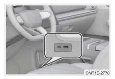
USB port is located on the lower front part of auxiliary fascia console.
