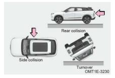
The driver airbag, front passenger airbag and driver knee airbag (if equipped) will usually not deploy if the vehicle is involved in a side or rear collision, if it rolls over, or if it is involved in a low-speed frontal collision.
