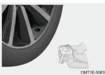
Step 2: Shake the automatic tire filler well before use, and then tear off the safety belt of the junction valve;
