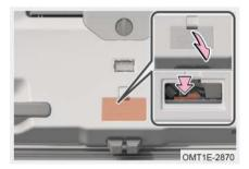
Back door cannot be opened when battery is depleted or under similar conditions. In this case, the back door can be opened with emergency device switch.
