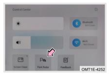
When vehicle is in READY state, slide down from the top right edge of the audio system screen, click parking radar button, parking radar system turns on; when shift lever is not in R, click parking radar button again to exit.
