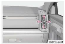
Move left/right side outlet adjustment lever up, down, left or right by hand to adjust direction of airflow.
