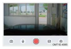
The driving recorder is connected to head unit through Wi-Fi and is displayed and operated on head unit. Click driving recorder application to enter the real-time screen of it. Swipe inwards from the left/right edge of the screen to return.
