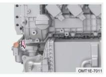
With the engine stalling and cooled down, check the oil level with the dipstick.
