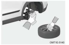
Step 1: Remove any attachments from mounting surface. Make sure wheel hub well contacts with wheel surface, and install spare tire;
