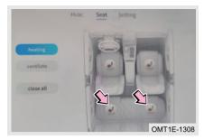
Method 1: After starting the vehicle, click rear seat heater button by air conditioning display screen - seat heating, it is 3-level heating (3 indicators on). Each time the switch is clicked, the heating level is lowered one level. Click it the fourth time to turn off the seat heating.
