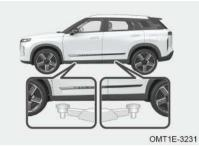
Make sure that the vehicle is on the correct jacking point to avoid damage to high/low voltage cables or power battery when the vehicle is lifted.
