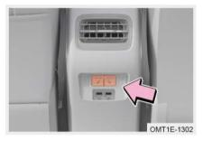
Method 2: After starting the vehicle, press the rear seat heater switch. it is 3-level heating (3 indicators on). Each time the switch is pressed, the heating level is reduced by one level. Press it the fourth time to turn off the seat heating.
