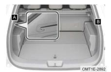
Pull the luggage curtain to the slots of point A and point B to secure it, and confirm if it is secured properly.
