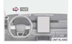
When head up display is turned on, a virtual image is formed in front of driver's field of vision to display the corresponding vehicle speed, driving mileage and other information.
