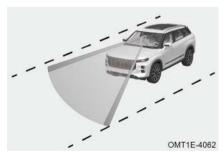
When vehicle speed is no less than 50 km/h and lane line is recognized, ELK-ot enters standby status.
