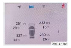
When the driving speed of vehicle is higher than 30 km/h and the continuous driving time is more than 45 s, the instrument cluster can display the tire pressure and temperature values in real time.
