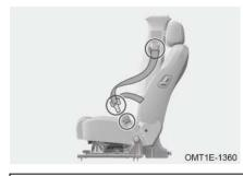
Check seat belts regularly for cuts, fraying, loose and stretched belt (such as after a traffic accident) If the seat belt is damaged, please contact authorized service station for inspection and repair immediately.
