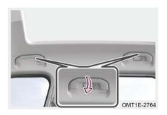
Assist grips are installed above front passenger door and both rear passenger doors respectively.
