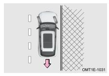
If there is a curb on the roadside, turn the steering wheel to the left to ensure that the rear part of the front right wheel is close to or against the curb, to prevent the vehicle from sliding back down the slope, then apply the parking brake.
