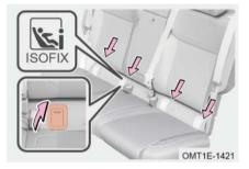
Step 1: Locate the ISOFIX anchorage; Please adjust the second row seat back angle to the front gear.
