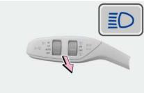
Pull headlight combination switch towards the steering wheel and release it to flash the high beam lights once. At the same time, headlight high beam indicator in instrument cluster flashes once.
