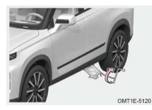
Step 4: When the notch of jack contacts correct jacking-up point, fit jack rocker into jack, and then fit wheel bolt wrench into jack rocker, and turn the wheel bolt wrench clockwise to jack up the vehicle;
