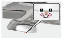
Before driving at night, adjust the inside rear view mirror lever to the anti-glare position, which can reduce the reflected light from the headlights of vehicles behind.
