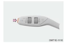
Spray mode: Shortly press the left button of wiper switch, the wiper will stop after wiping once; Press and hold the left button of wiper switch, the front washer sprays water, and front wiper operates simultaneously. Front washer will stop operating when the switch is released, the wiper will wipe 3 cycles at low speed, and operate one cycle then stop after a few seconds.
