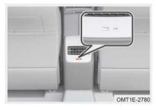
Rear USB port can be used for charging the electrical equipment with low power, such as phone etc.
