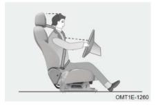
The shoulder belt should be over the center of the shoulder and close to the chest, kept away from the neck, the lap belt should lie over the hips instead of stomach.
